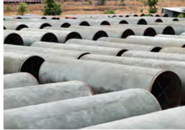
Gunnitted MS Pipes Stockyard
